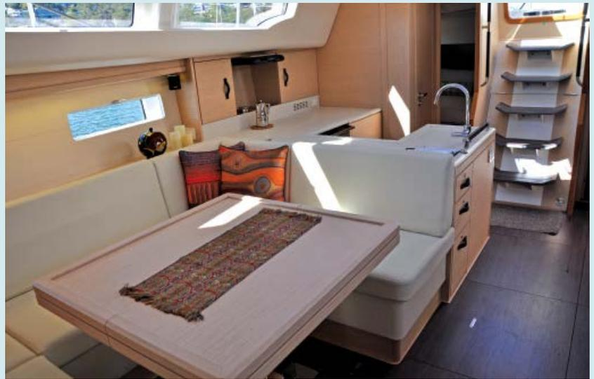
**ABOVE:** With the aisle offset to port it allows a large lounge area, note the utility room aft of the galley.
